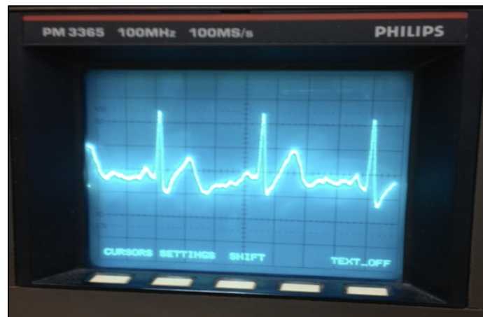
Figure 34: ECG signal measured at the fingertips using Plessey sensors
