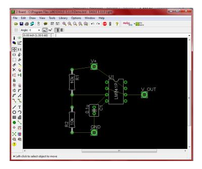
The RATSNEST command will clean up the airwires, reconnecting them to the shortest path between components. Press RATSNEST. Note that the airwire for the positive op-amp input shifted to a shorter path.
