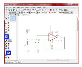
Repeat, using the name "V+" for the unconnected nets on R1 and pin seven.
