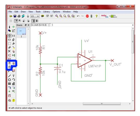
The REPLACE command (located between ADD and VALUE) can be used to swap equivalent parts such as resistors with different footprint sizes without removing them from the schematic and disconnecting any associated. Do not replace anything at this time.
