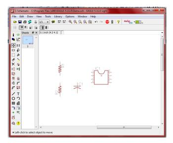
IC1 has the correct footprint for an IC but it does not have a desirable schematic symbol. Select the DELETE command and left click IC1.
