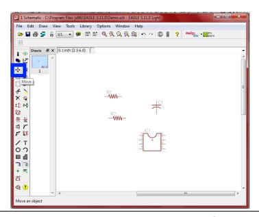
Repeat this so R1 and R2 are vertically aligned and C1 is parallel of R2.
