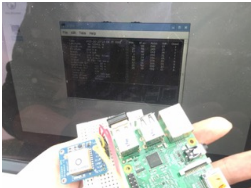
Fig 22 . GPS Data Obtained on Raspberry Pi Desktop
