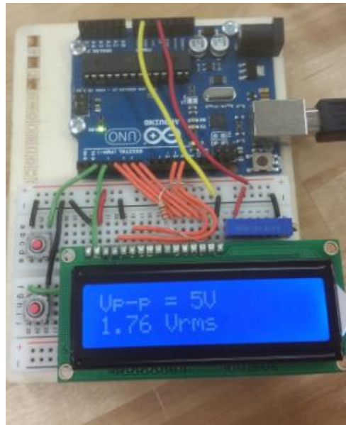
Figure 20. Stage 1 Prototype – Arduino Uno, LCD, and buttons
