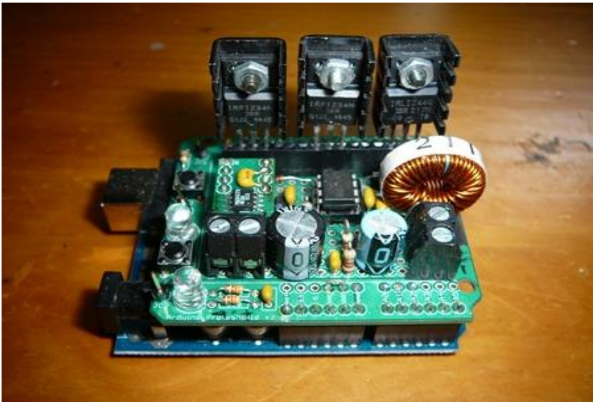
An example of a PCB-based Boost Converter 2
