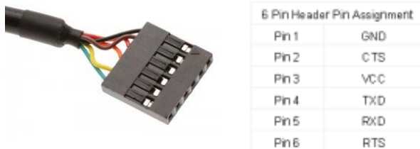
Figure 1: 6-Pin RS-232 Cable and Pin Assignment
