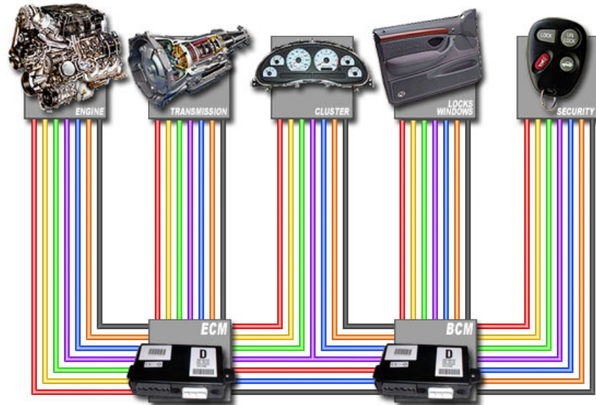
Vehicle Wiring: conventional multi-wire looms
