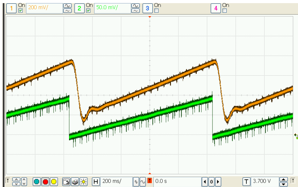
Output (Yellow) Compared to Input (Green) in Butterworth Filter Test
