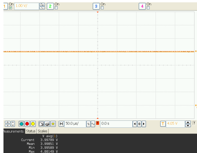
Output of the Bessel Lowpass Filter at 75% Duty Cycle
