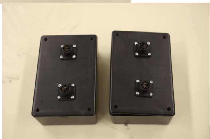
PICTURE 4 TRANSMITTER AND RECEIVER SHOWN SEALED.
