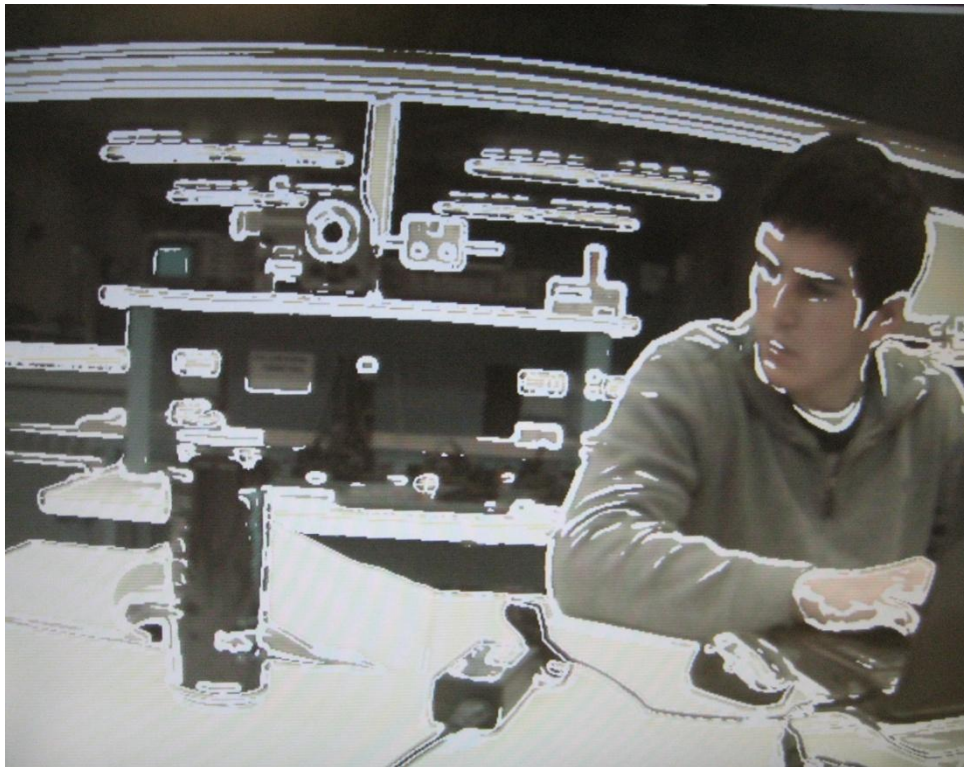
Figure 53: Threshold at 220- Set too High
