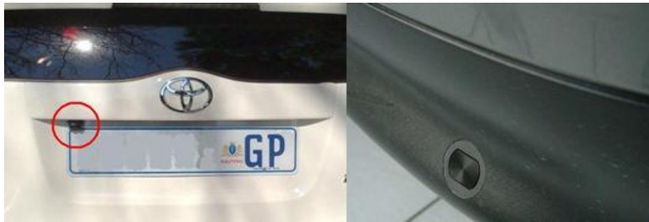
Figure 2: Rear-View Camera (Left) and Ultrasonic Sensor on rear bumper (Right)
