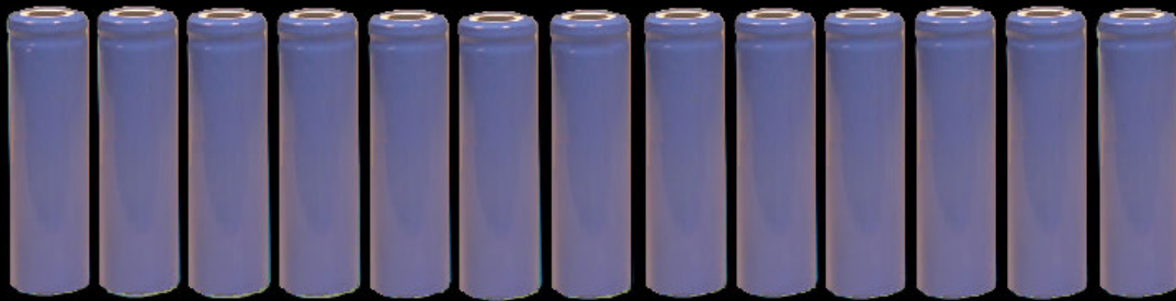
Figure 7. Due to the poor selection of 48.1V Li-ION batteries on the commercial market, we will be constructing our own battery from 13 individual Li-ION cells. This battery will include a Protection Circuit Module (PCM) which will prevent overcharge and discharge and balance the energy in the individual cells.
