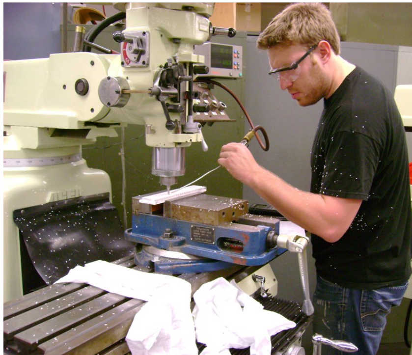
Figure 1. Milling of the Bearing Channels
