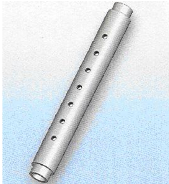
Figure 6.9: Conceptual design of a rotating sub-chamber.
