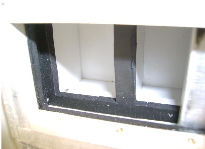
Figure 6.20: Viton seal of inner sub-chambers. Note the fraying of the center piece of Viton.
