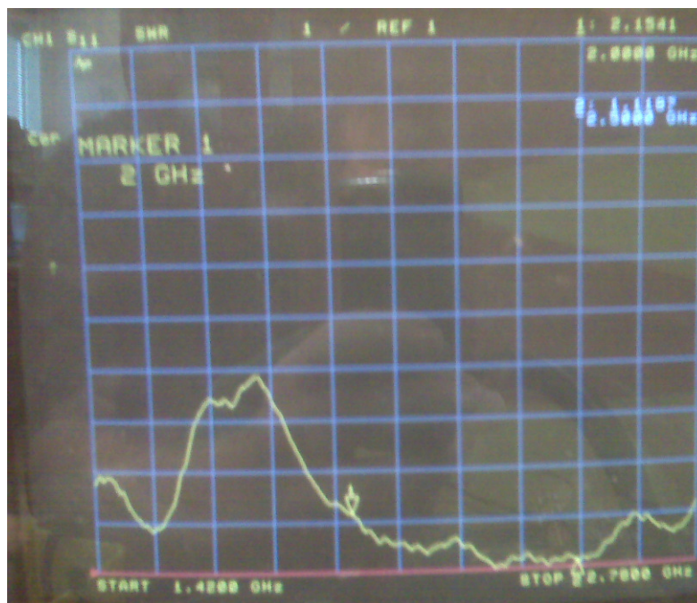
Figure D.3: VSWR of LTSA "B" from 1.4GHz to 2.8GHz
