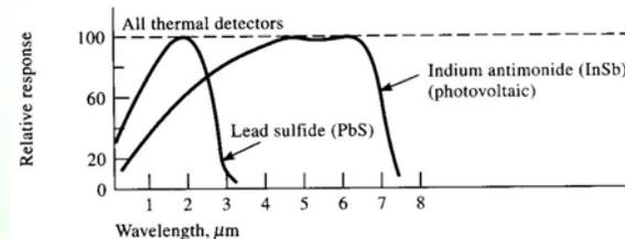
(c) spectral sensitivity of photon and thermal detectors
