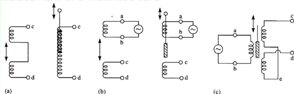
**Figure 2.6** Inductive displacement sensors (a) Self-inductance. (b) Mutual inductance. (c) Differential transformer.
