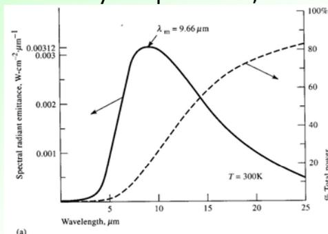
(a) spectral radiant emittance & % of total energy
