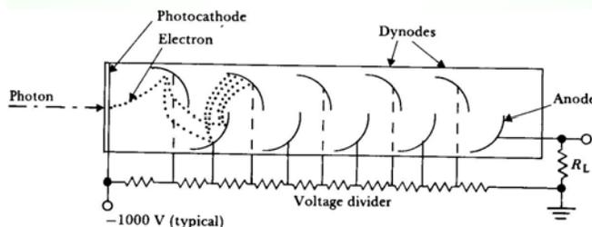
**Figure 2.21 Photomultiplier** An incoming photon strikes the photocathode and liberates an electron. This electron is accelerated toward the first dynode, which is 100 V more positive than the cathode. The impact liberates several electrons by secondary emission. They are accelerated toward the second dynode, which is 100 V more positive than the first dynode. This electron multiplication continues until it reaches the anode, where currents of about  $1\ \mu\text{A}$  flow through  $R_L$ .
