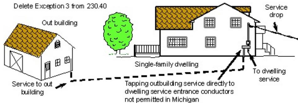
**Figure 1** Exception 3 of NEC® 230.40 was deleted from the MEC. It is not permitted to directly supply an outbuilding from a single-family dwelling service drop or lateral.
