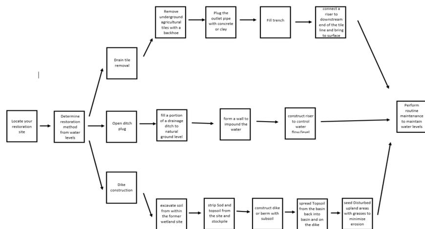
Figure 2. Flowchart detailing the steps involved in a standard wetland restoration process including site determination, choosing restoration method (Open ditch plugging, underground drain tile removal, or dike construction), and continued maintenance of the restored wetland site post restoration
