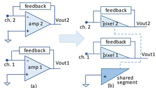
Fig. 2. (a) A traditional 2-channel amplifier and (b) a 2-channel amplifier using a shared-segment configuration.
