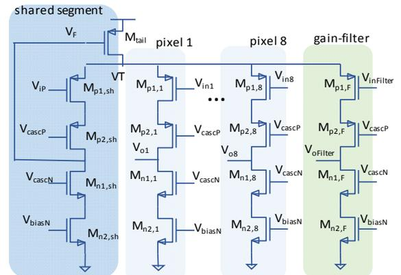
Fig. 5. Schematic of a shared telescopic OTA.
