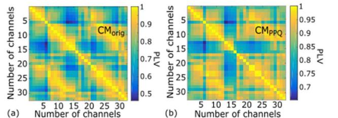
Fig. 7. CMs of 32-channel ECoG data in alpha band (a) unquantized original data and (b) PPQ decimated data which achieves 89.1% accuracy compared to  $CM_{orig.}$ .
