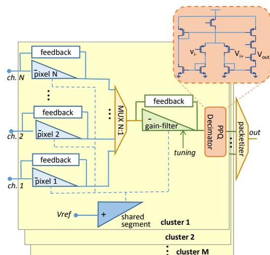
Fig. 3. Neural recording system for  $n = N \times M$  channels with hardware resource sharing. The inset shows the schematic of the 1-bit PPQ quantizing comparator.
