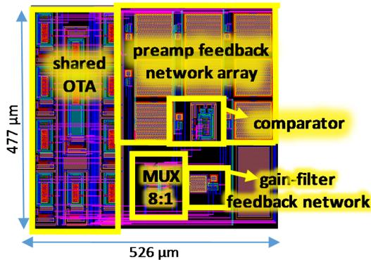
Fig. 6. Layout of 8-channel neural amplifier with tunable filter and data decimator (comparator).
