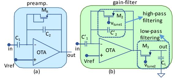
Fig. 4. (a) Preamplifier with capacitive feedback, and (b) tunable filter and gain stage.
