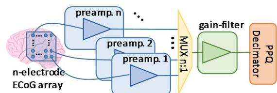
Fig. 1. Illustration of an  $n$ -channel neural recording system.
