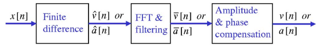
Fig. 3 The three-stage data processing algorithm, applicable to both the forward difference method and the central forward method
