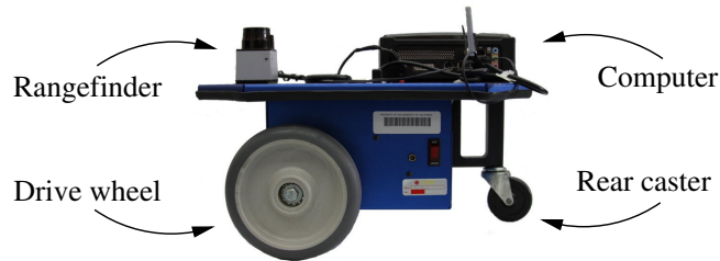
Figure 4.10: Erratic mobile robot with URG-04LX laser rangefinder.
