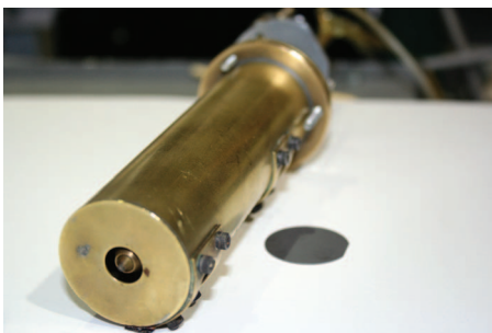
FIG. 2. (Color) Photograph of the overall microwave re-entrant cavity applicator adjacent to a 1 in. silicon wafer.
