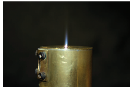
FIG. 3. (Color) Photograph of the re-entrant cavity showing the microwave applicator exciting a pre-mixed flame.
