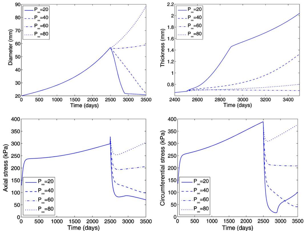
Fig. 5 AAA diameter, thickness, the circumferential component, and the axial component of the stress at the middle point of the wall with respect to time for different final intrasac pressure  $P_\infty$
