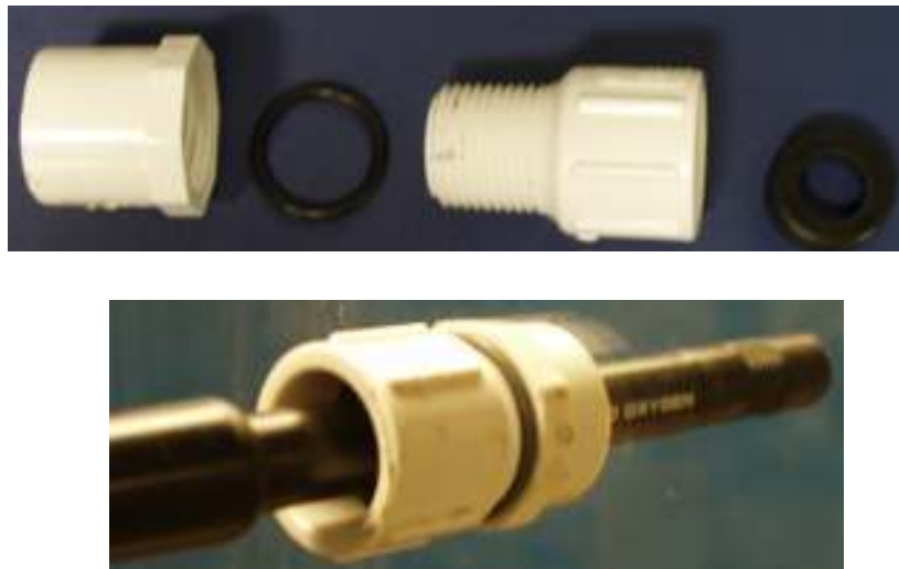
Figure 4. Sensor seal. Upper panel. Individual components of the sensor seal. From left to right: reducer bushing ( 3/4" \times 1/2" ), O-ring washer ( 3/4" ), reducing coupling ( 1/2" ), rubber grommet (provided with dissolved oxygen sensors). Lower panel. Sensor inserted in seal.
