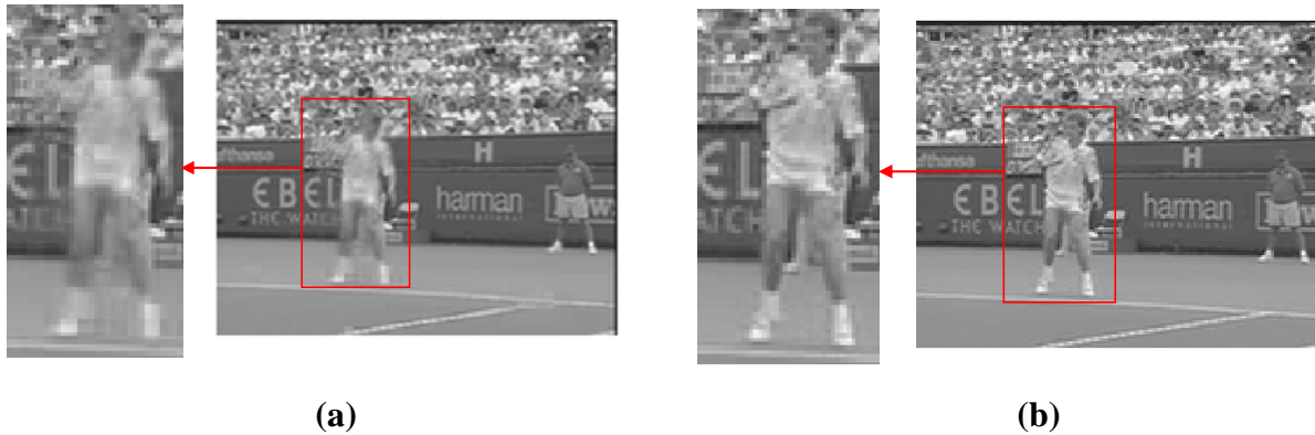
Figure 9: Stefan-QCIF, frame 36 of (a) Interpolation scheme (452 Kbps) and (b) Proposed codec (388Kbps)
