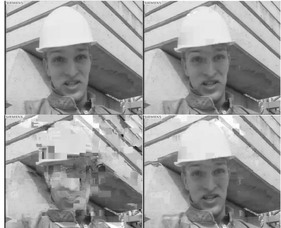
Figure 3 Clockwise an instance in the foreman Sequence for L=12 RS code, L=12 PRS – 1 code optimized for p=0.11 , L=13 PRS – 1 code optimized for p=0.11 , L = 13 RS code.
