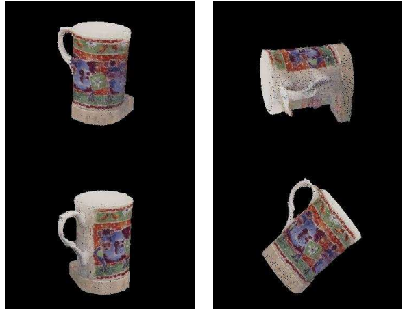
Figure 5 The generated synthetic images resulting from re-projecting the VM5c back to image planes for new camera viewing positions that are different from those for the original images.
