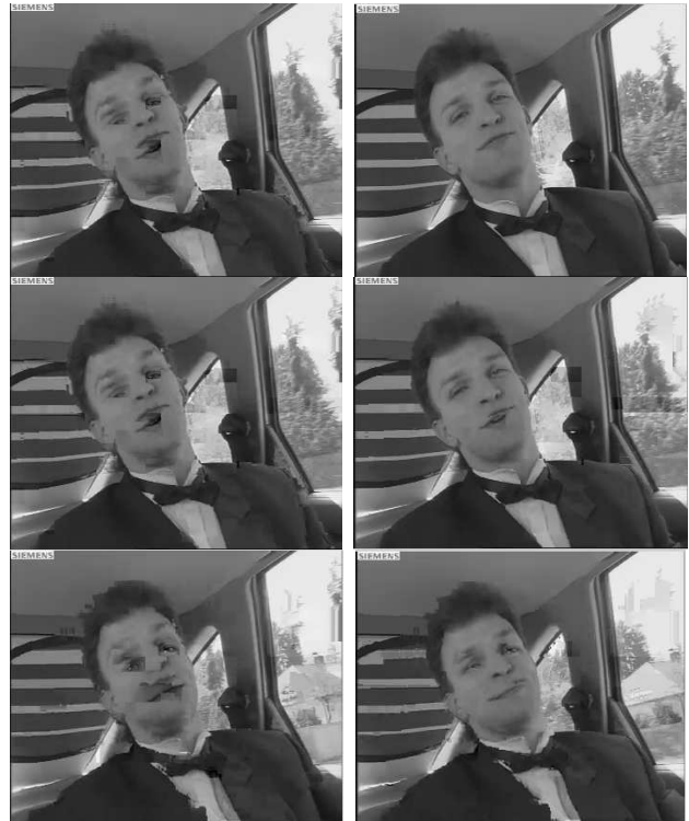
Figure 6 Comparison of carphone over (wired) Internet, left column: frames 354, 357, 370 from a rs-based scheme, right column: frames 354, 357, 370 from a prs-based scheme.
