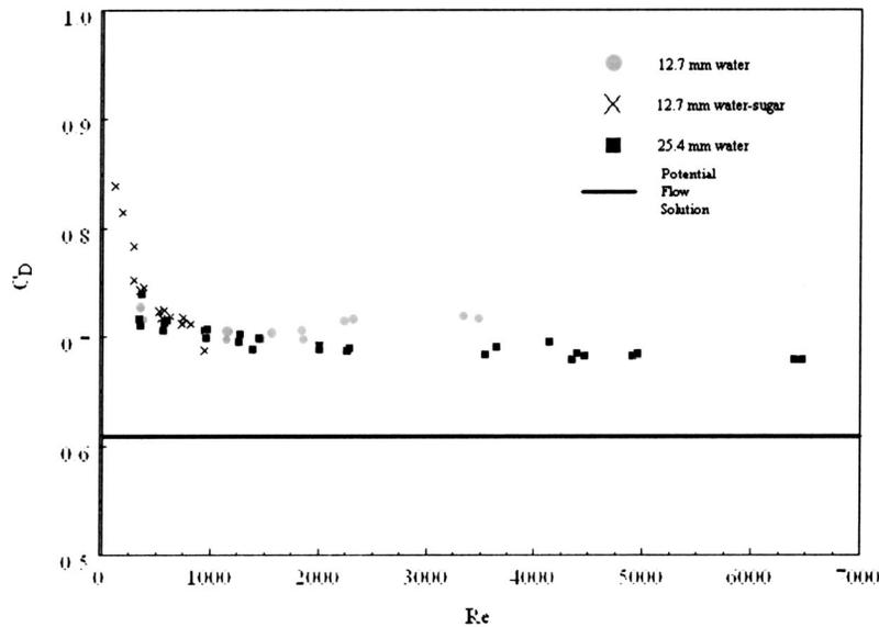
Fig. 4 Distribution of discharge coefficient  $C_D$  as a function of Re in jets with two different nozzle configurations:  $[w, t_N/w, B_N/w]$  [12.7 mm, 1, 21.7] and [25.4 mm, 0.5, 10.8]. Note that two different working liquids were used for the jet with  $w = 12.7$  mm. See Fig. 2 for the corresponding estimates of uncertainty in  $C_D$ . The solid line represents the potential flow solution for  $C_D$ .
