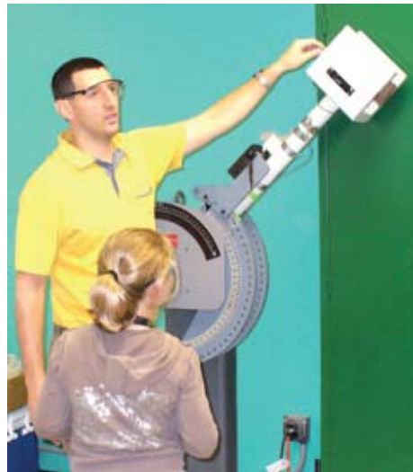
Carl Boehlert, associate professor of chemical engineering and materials science, demonstrates how to use a Charpy Impact Tester as part of a SEMED program for K-12 students. Isabella Davids of Hazel Park, Mich. looks on. See story on page 1.
