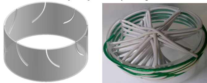
Fig. 3 Wound Impeller; left: Simple Support Structure; right: Matching Manually Wound Model with 2 Fibers that are approx. 10 X Enlarged for Demonstration (Fig. 5, in 1 st row – 2 nd Pattern from left)
