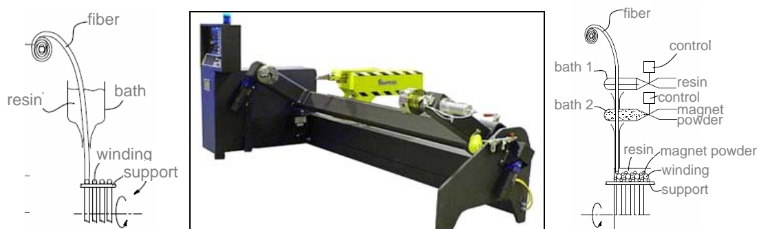
Fig. 2 center: Example of Multiple Axis Winding Machine ( www.mccleananderson.com ) left: Fiber Wetting with one Bath, right: Controlled Alternative Fiber Wetting with two baths
