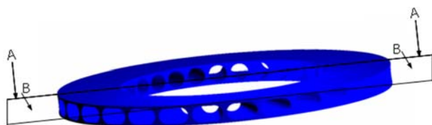
Fig. 13 Radial wave rotor with rounded cross-sectional channels
