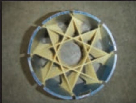
This is one of the first woven turbo wheels with an integrated induction motor that spins up to 6000 rpm.
