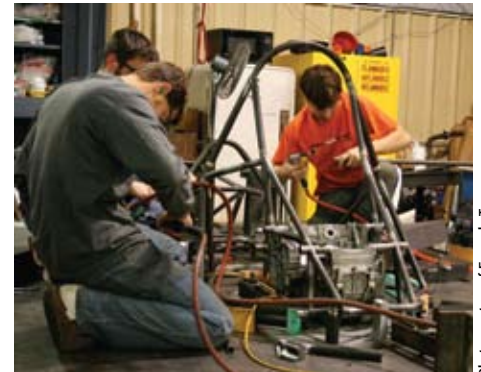
MSU Formula Racing Team members (from left to right) Scott Williams, Drew Darling, and Paul Strefling grind tubing for Car 51's chassis.
