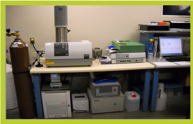
New Netzsch LFA 457 Laser Flash System installed and operational in C24
