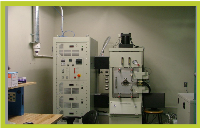
Pulsed Electric Current Sintering (PECS) System installed in C24 ERC.
