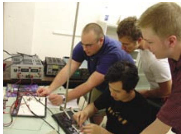
ECE students, left to right, Anthony Cerri, Zheng Chen, Jason Malinak, and Christopher Ziel, are testing a two degree-of-freedom robotic arm made of IPMCs.
