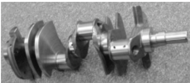
Figure 1: Crankshaft used in the experimental engine with two CPVAs attached, one at the first and last counterweight area of the crankshaft.
