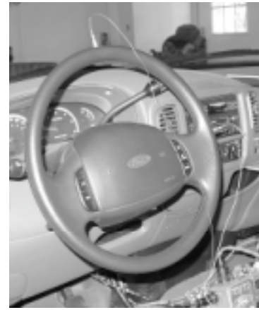
Figure 4: Accelerometer mounted at the 12-o'clock positions on the steering wheel.
