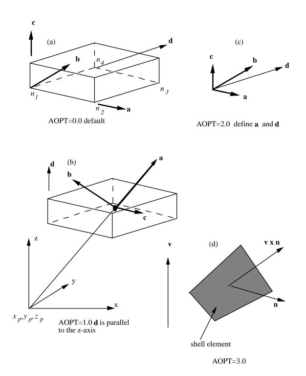
Figure 23-1. Options for determining principal materials axes: (a) AOPT = 0.0, (b) AOPT = 1.0, and (c) AOPT = 2.0.
