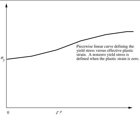
Figure 20-4. Effective stress versus effective plastic strain curve.
