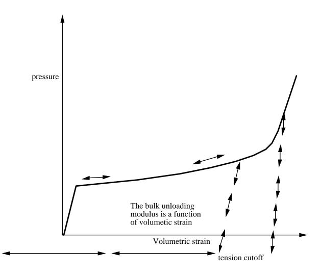
Figure 21-1. Pressure versues volumetric strain curve for equation-of-state form 8 with compaction. In the compacted states the bulk unloading modulus depend on the peak volumetric strain.
