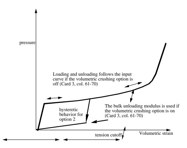
Figure 22-3. Volumetric strain versus pressure curve for soil and crushable foam model.
