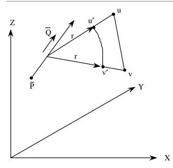
Figure 6-9. Cylindrical surface.
