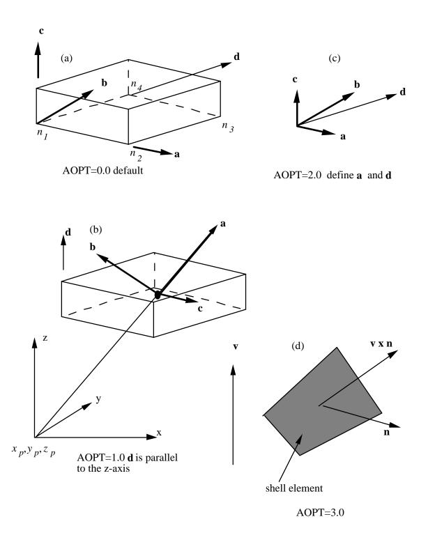
Figure 19-1. Options for determining principal materials axes: (a) AOPT = 0.0, (b) AOPT = 1.0, and (c) AOPT = 2.0.
