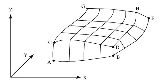
Figure 6-1. Mapping from index space to object space.
