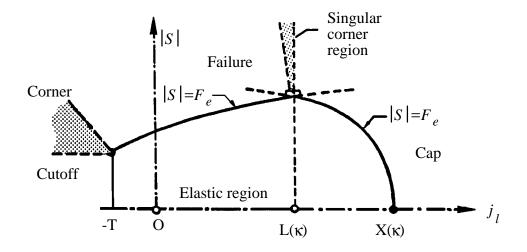
Figure 19-5. The yield surface of the two-invariant cap model in pressure/J<sub>2</sub>-deviator space.  $f_1 = 0$ ,  $f_2 = 0$ , and  $f_3 = 0$ , denote the failure envelope, the hardening cap surface, and the tension cut-off surface, respectively.
