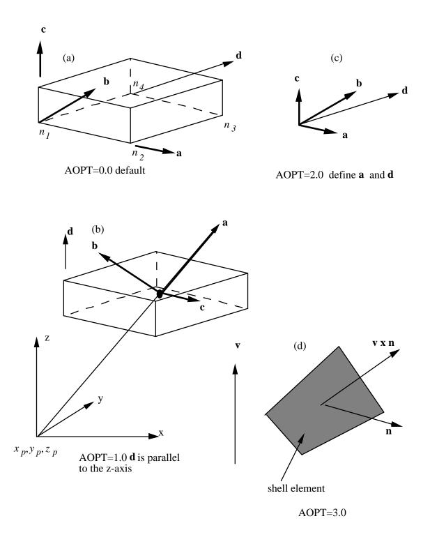
Figure 22-1. Options for determining principal materials axes: (a) AOPT = 0.0, (b) AOPT = 1.0, and (c) AOPT = 2.0.
