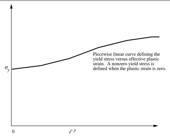
Figure 19-4. Effective stress versus effective plastic strain curve.
