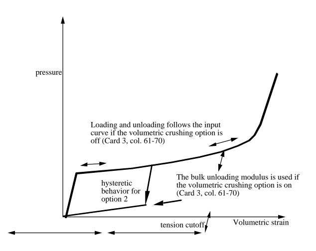
Figure 19-3. Volumetric strain versus pressure curve for soil and crushable foam model.
