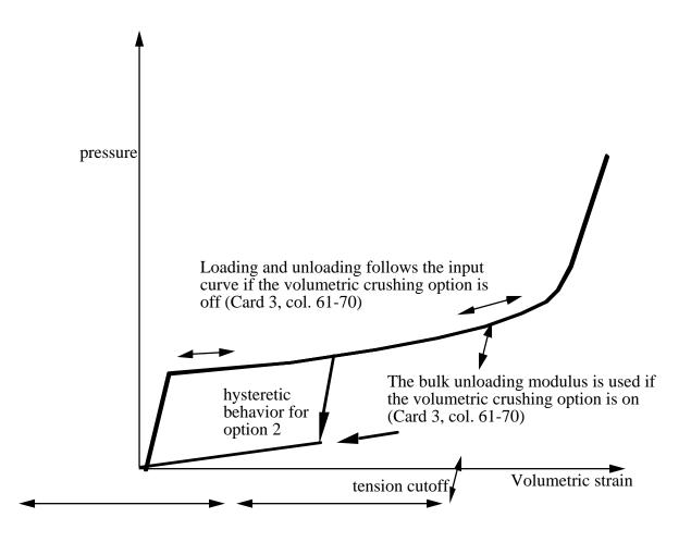
Figure 23-3. Volumetric strain versus pressure curve for soil and crushable foam model.
