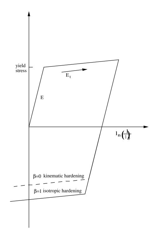
Figure 23-2. Elastic-plastic behavior with isotropic and kinematic hardening where  $l_0$  and l are undeformed and deformed length of uniaxial tension specimen.
