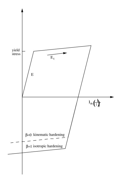
Figure 20-2. Elastic-plastic behavior with isotropic and kinematic hardening where  $l_0$  and l are undeformed and deformed length of uniaxial tension specimen.
