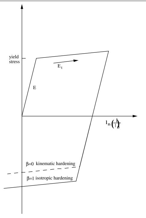
Figure 19-2. Elastic-plastic behavior with isotropic and kinematic hardening where  $l_0$  and l are undeformed and deformed length of uniaxial tension specimen.
