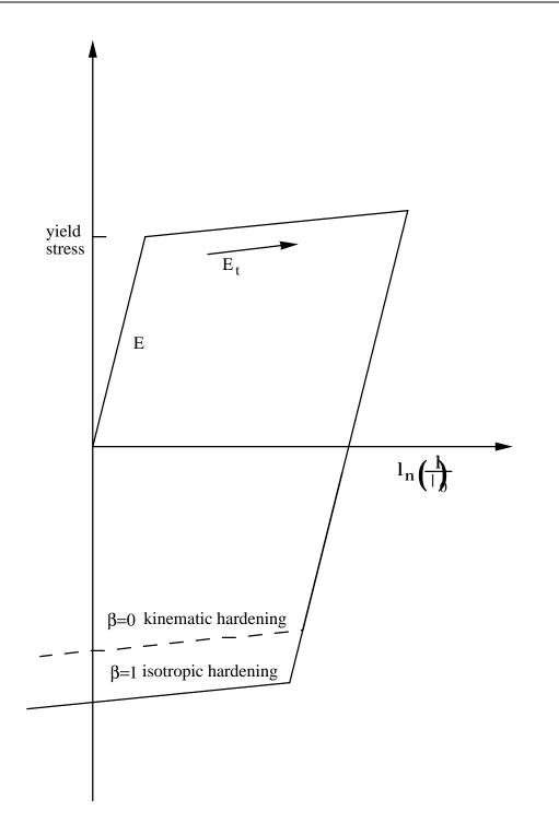
Figure 22-2. Elastic-plastic behavior with isotropic and kinematic hardening where  $l_0$  and l are undeformed and deformed length of uniaxial tensions specimen.
