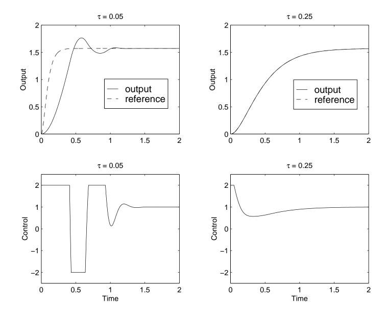
Third Approach: Plan a trajectory  $(r(t), \dot{r}(t), \dots, r^{(\rho)}(t))$  to move from  $(0, 0, \dots, 0)$  to  $(\bar{y}, 0, \dots, 0)$  in finite time T Example:  $\rho = 2$
