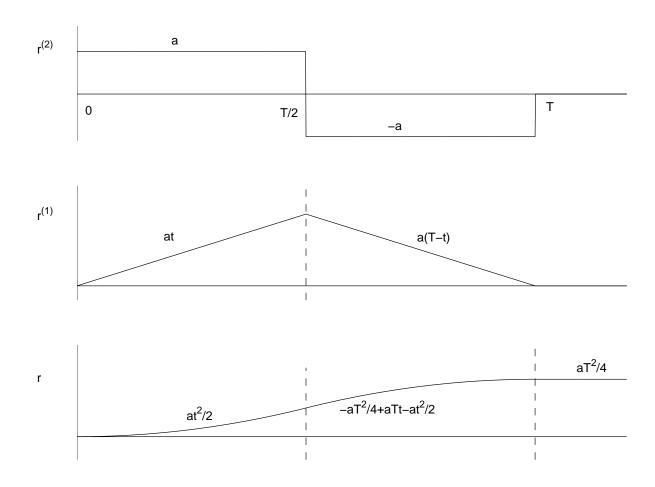
$$r(t) = \begin{cases} \frac{at^2}{2} & \text{for } 0 \leq t \leq \frac{T}{2} \\ -\frac{aT^2}{4} + aTt - \frac{at^2}{2} & \text{for } \frac{T}{2} \leq t \leq T \\ \frac{aT^2}{4} & \text{for } t \geq T \end{cases}$$
