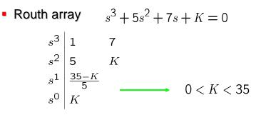
If K=35, oscillation frequency is obtained by the auxiliary equation
