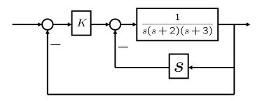
Determine the range of K and a that stabilize the closed-loop system.
