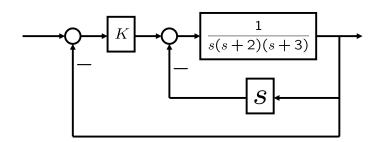
Determine the range of K and a that stabilize the closed-loop system. Example 2 (cont'd)
