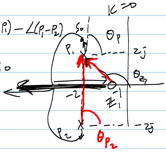
$$CE \Rightarrow 1 + KL(s) = 0 \quad L(s) = -\frac{1}{k} \quad \angle \pm 180^\circ$$
