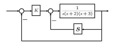
Determine the range of K and a that stabilize the closed-loop system. Example 2 (cont'd)
