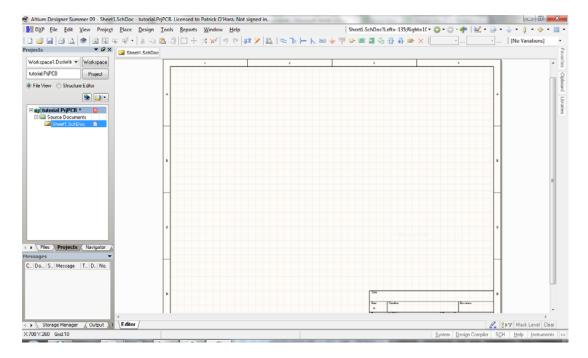
To rename the schematic file go to **File>Save As** and save the file in the same directory as the project. If the schematic sheet is not automatically added to the project you can drag the file in the Project panel from free documents to the project. Before starting creating the circuit several schematic options may be set by going to **Design>Document Options**. Here we will only change the Standard Style to A4.
