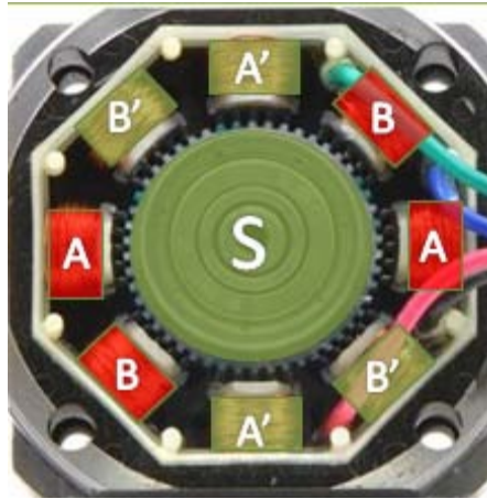
Figure 3. Stepper Motor Innards
