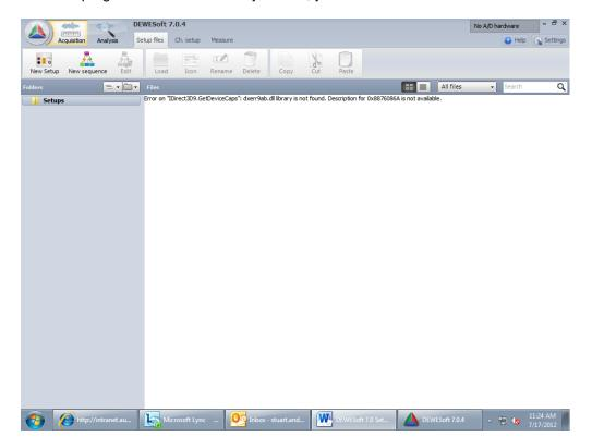
3. From here, click on the button located on the tab ribbon on near the top named "New Setup".
