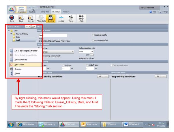
26. Next we will want to setup up the "Measure" tab on the top ribbon bar.
