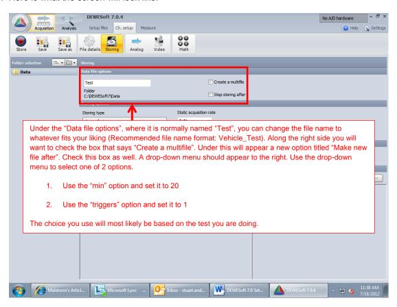
21. The screen below should look like this after completing the above tasks. Next are the "Storing options" and "Trigger setup" which are underneath the "Data file options".
