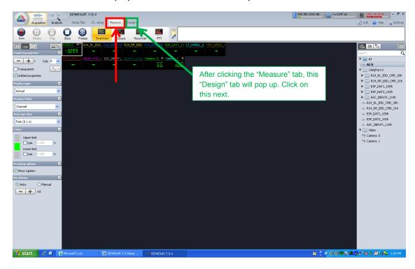
27. From here you see this screen. This is where you will design layout and messages you would like to see displayed as well as the picture for the cameras being used for the test. The next few screenshots will step you through the process of creating your layout.
