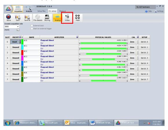
11. Now at this point you should see the cameras that you have attached. Depending on if you are using 2 or 4 cameras, this next part will be slightly different. First under "Store options", change the drop-down bar to the option of "fast on trigger, but slow otherwise" (Red).
