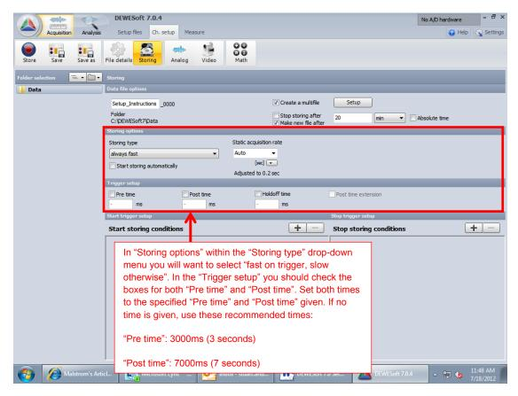
22. The next step is the "Start trigger setup". Under that title you will need to configure the "Start storing conditions". Use the plus button to the right to add a condition and then click the "Setup" button on the condition.
