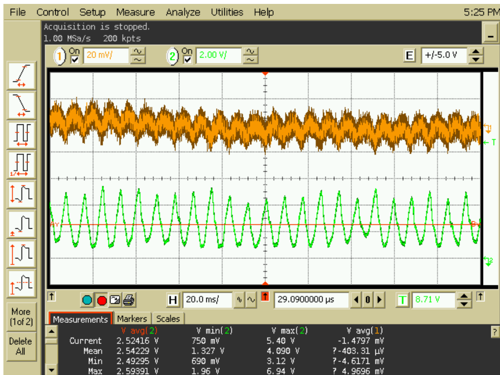
Figure 13 – Complete system gain. Note the visible noise on channel 1 is artificial – it is due to the oscilloscope probe's picking up noise and is not actually present in the circuit.
