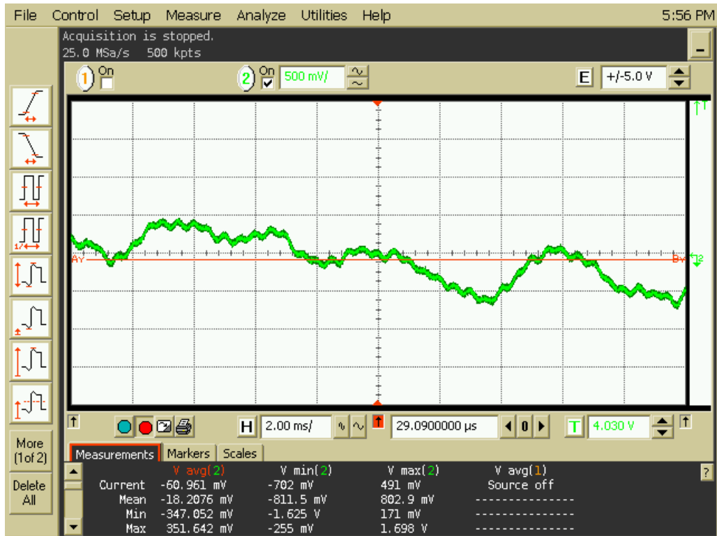
Figure 6 – Amplifier picking up 2000 Hz tone from speaker.
