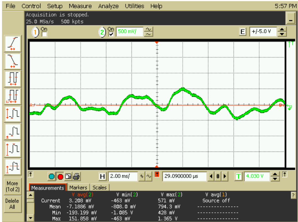
Figure 4 – Amplifier picking up 500 Hz tone from speaker.
