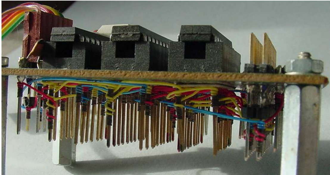
Figure 3: Wire-wrap prototype. Note 0.1” spaced 0.025” square post headers at right.
