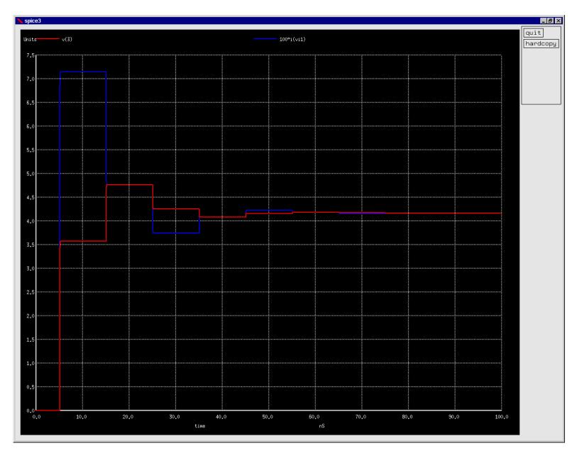
Fig. 5: Plot of voltage and current at midpoint of transmission line shown in Fig. 4 using Spice3 with the input file shown in Table 4.
