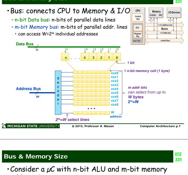
address bus \*\*generally, #ALU bits = #bits per memory cell\*\*
