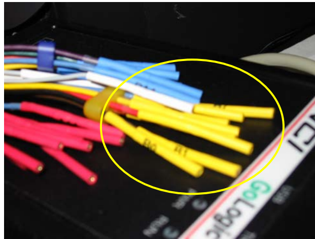
Figure 2. Female connectors of Logic Analyzer
