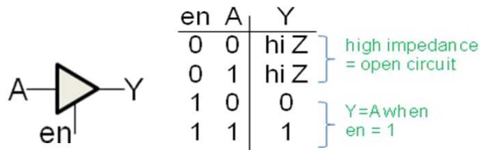
Tri-state buffer gate symbol and truth table.
